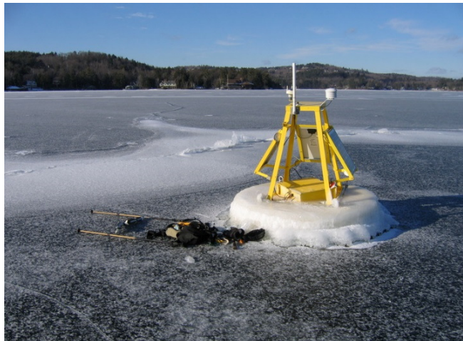
Figure 1. Water quality monitoring buoy frozen into Lake Sunapee N.H. USA. For many winters the buoy performed well, however in one year it was damaged at the time of ice loss. Photo credits: Midge Eliassen
